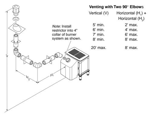
Figure 35 - Vertical Rigid Venting Configuration Using Two 90° Elbows with Two Horizontal Runs
